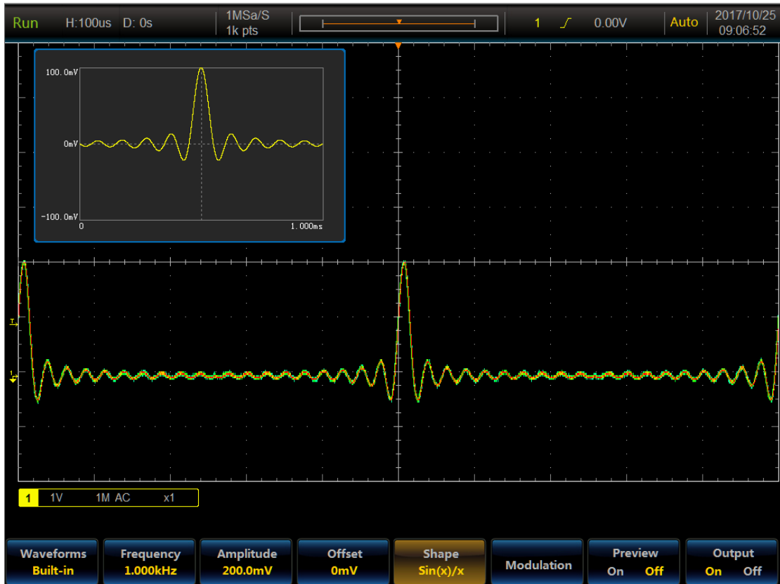
Built-in waveform output: SinC, Exponential Rise/Decay, Gaussian, Lorentz curve and haversine curve
