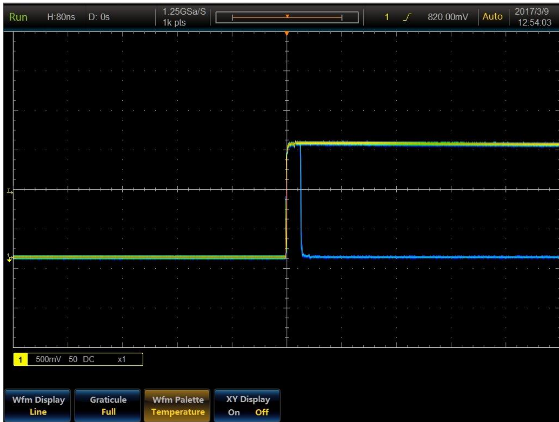
1000,000 wfms/s waveform capture rate, fast identification of contingency.
