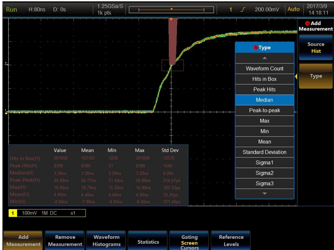
Horizontal histogram: to observe jitter and jitter distribution of signals.
